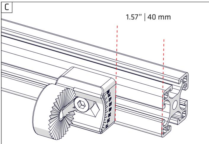
Tighten the bolts with full force. Ensure that you hold the long side of the Allen key in your hand as this enables you to exert greater force.
