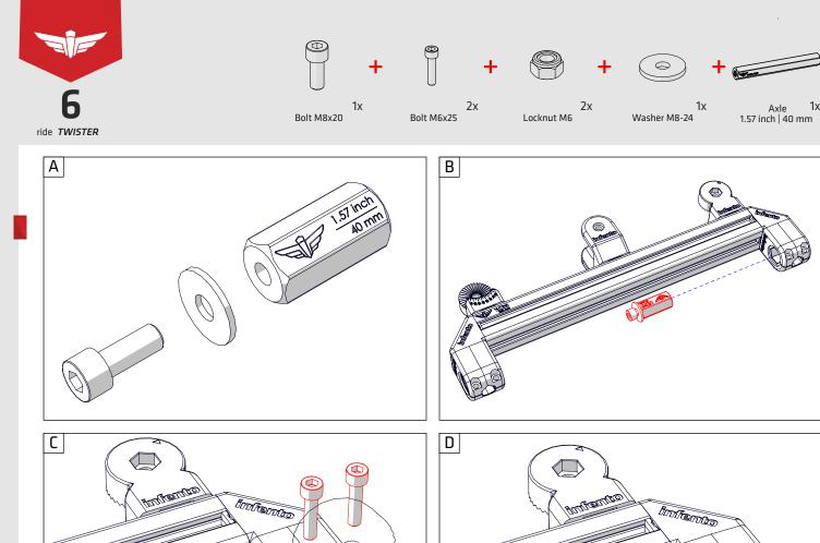
Leave a gap of at least 0.5mm when tightening the bolts.
