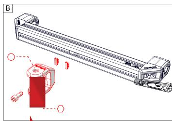
When tightening the bolt always check whether the profile nut remains perfectly straight in the slot. If this becomes crooked, you can push against the side of the profile bolt with the Allen key to correct this.
