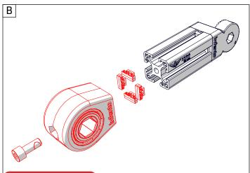
Use the Allen key handle so you can tighten the bolt well.
