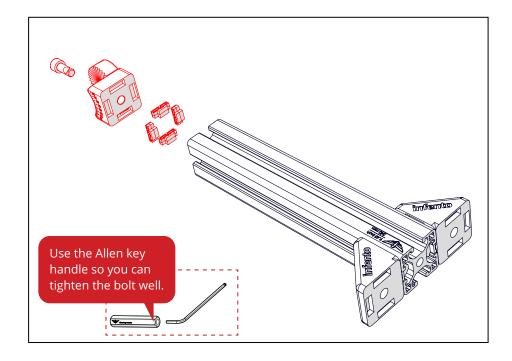
The positioning blocks are some of the smallest Infento parts but they are also some of the most important. They ensure that everything connects to each other properly. This prevents parts from twisting and coming loose when under pressure. Therefore, always use at least two positioning blocks per block.
