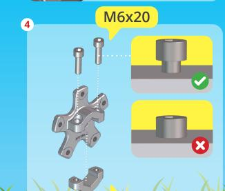
Clamping part WITH THREAD
