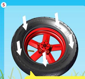
Pull the tire over the rim and inflate the tire to max 2 bar.
