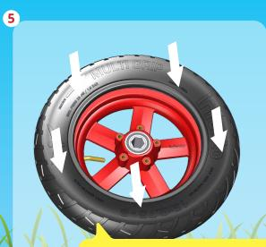
Pull the tire over the rim and inflate the tire to max 2 bar.
