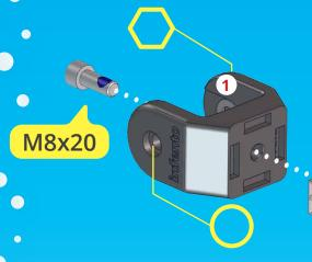
Add a small droplet of threadlock to secure the bolts
